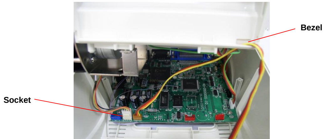
Fig. 16 Cutter module harness arrangement
