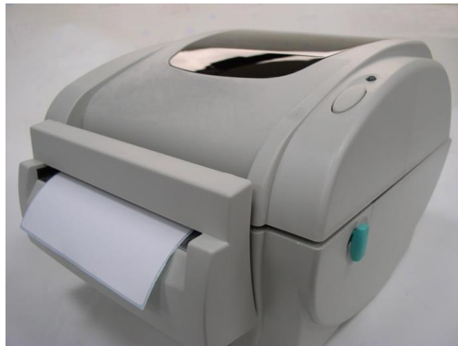
Fig. 19 Media installation in cutter mode completed
