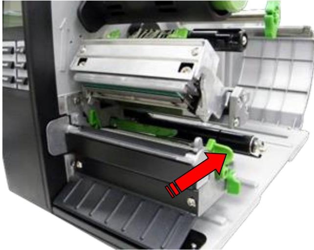
3. Install the ribbon onto the supply spindle.
