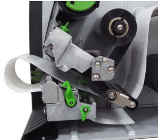
5. Wrap the label onto the internal rewind spindle and wind the spindle counter-clockwise 3~5 revolutions until the label is properly stretched.
