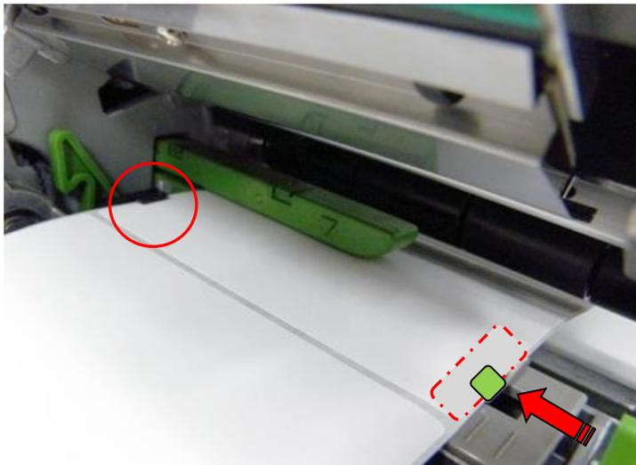
10. Close the print head mechanism. Make sure the latches are engaged securely.
