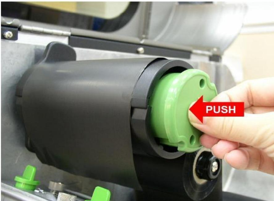
3. Slide/pull the used ribbon off the rewind spindle.
