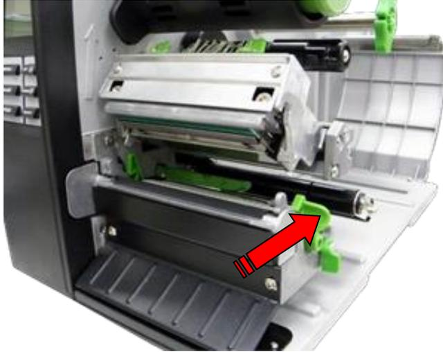
3. Move the label roll guard horizontally to the end of label spindle then flip down the label roll guard.
