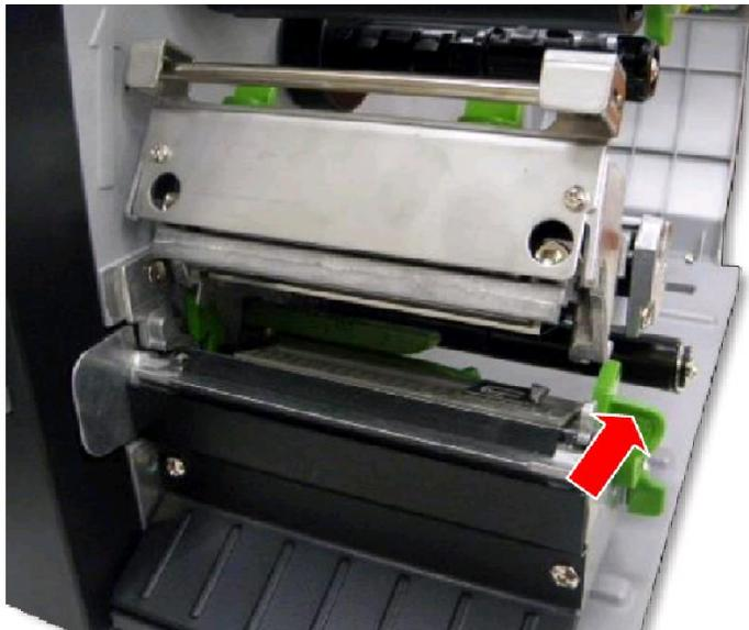
3. Move the label guard across the spindle and lay it down horizontally.
