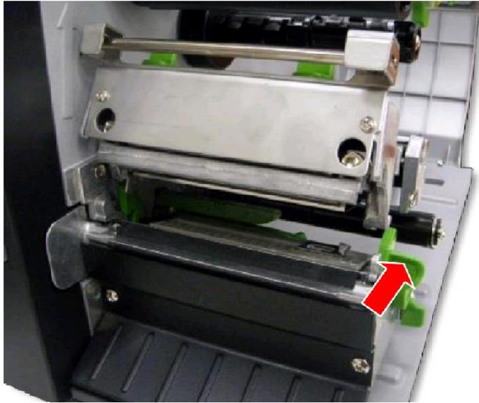
3. Install the ribbon onto the supply spindle.
