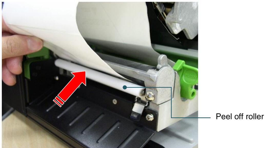
5. Feed label through mechanism.
