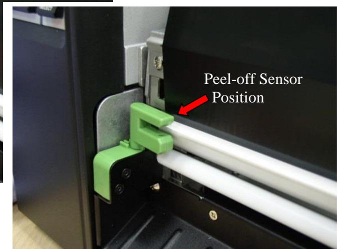
8. Label peeling will automatically start. Press the FEED button to test
