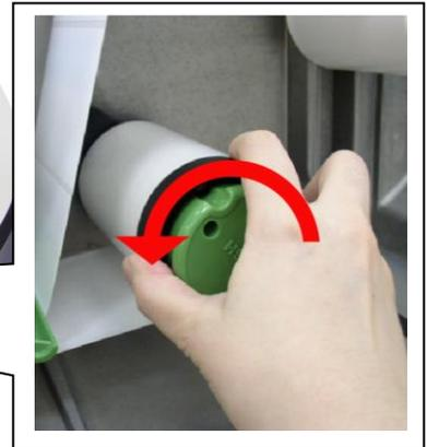
7. Lift up the peel-off roller release lever and close the print head mechanism. Move the peel-off sensor toward the paper exit chute.
