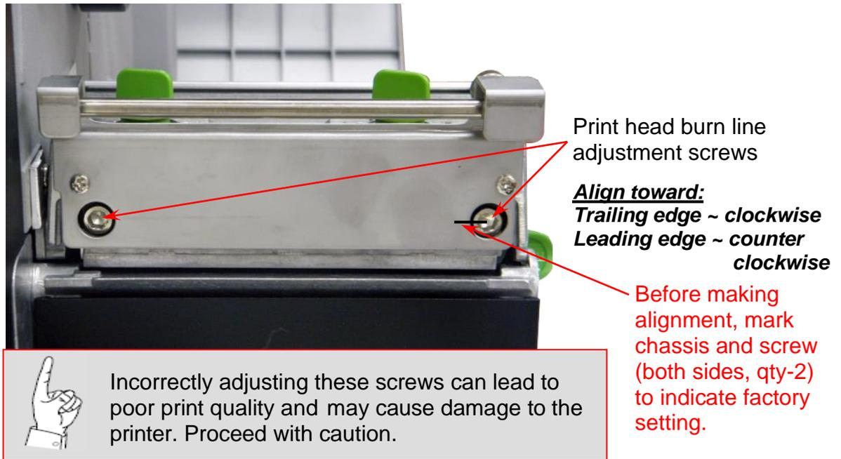
Before proceeding with burn line adjustment; verify print density, print head pressure adjustment, or z-axis alignments are properly adjusted. As a reference mark the chassis and screw(s) to indicate the factory setting, should it need to be restored.
