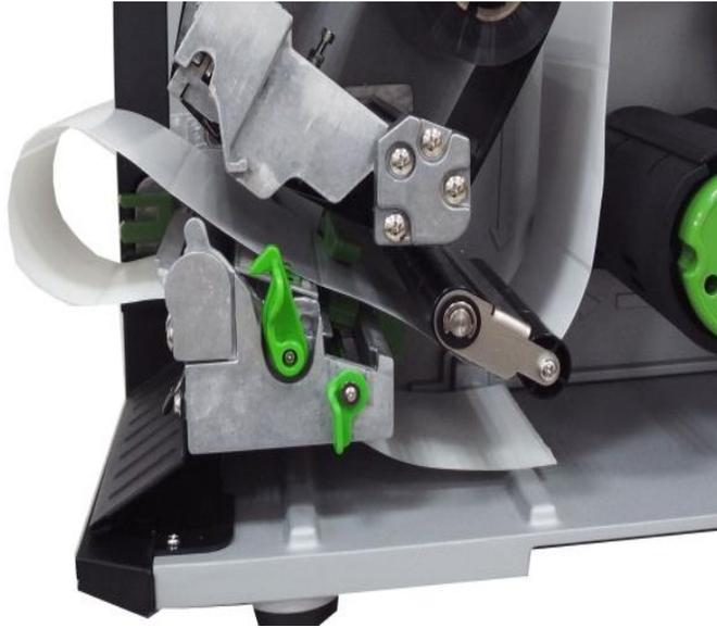
6. Wrap the label onto the internal rewind spindle and turn the spindle counter-clockwise 3 to 5 turns until the slack is removed and properly stretched.
