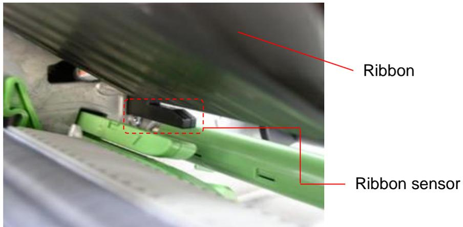
5. Wrap the ribbon onto the rewind spindle. Turn the spindle clockwise 3~5 complete turns. Verify the ribbon is properly stretched/flat without wrinkles.
