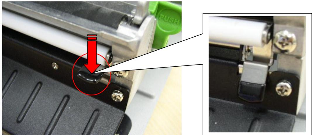
4. Feed the label between peel-off roller and platen roller.
