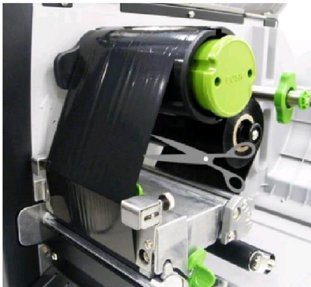
2. Push green button to release ribbon from the spindle.
