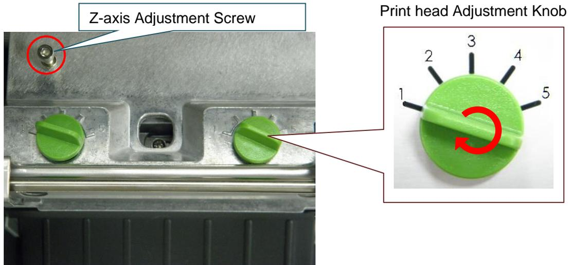
2. If the wrinkle on the printed label starts from the lower left side to upper right side, follow this adjustment procedure:
