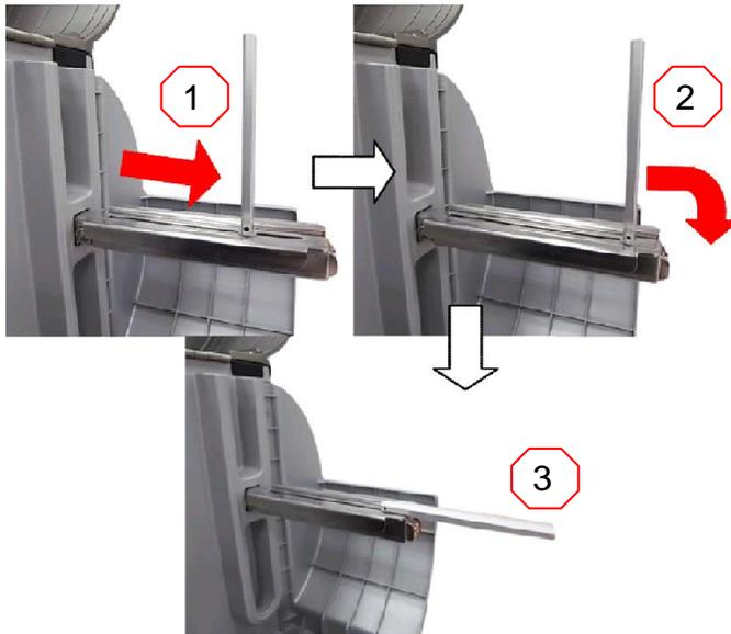
4. **NOTE:** The 3" label spindle can be removed to support a 1" core, by removing two screws.
