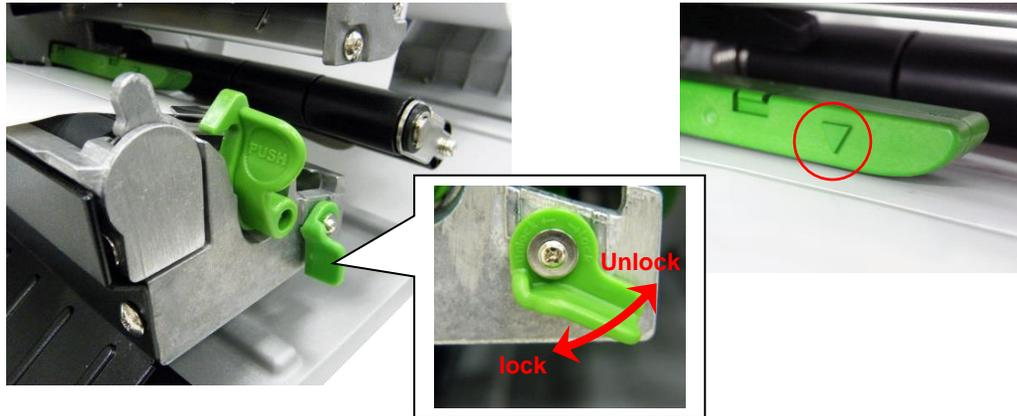
8. Adjust the label guides to fit the width of the media.
