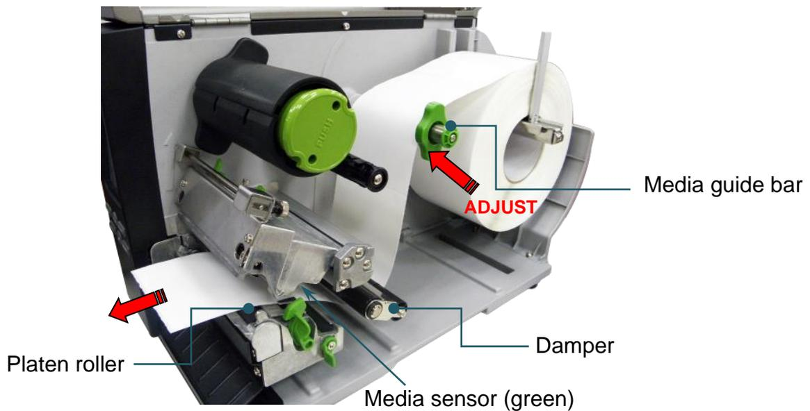
7. Unlock the media sensor to adjust. Align sensor (green triangle ▼ ) over label gap or black mark for proper sensing. After alignment re-lock sensor.
