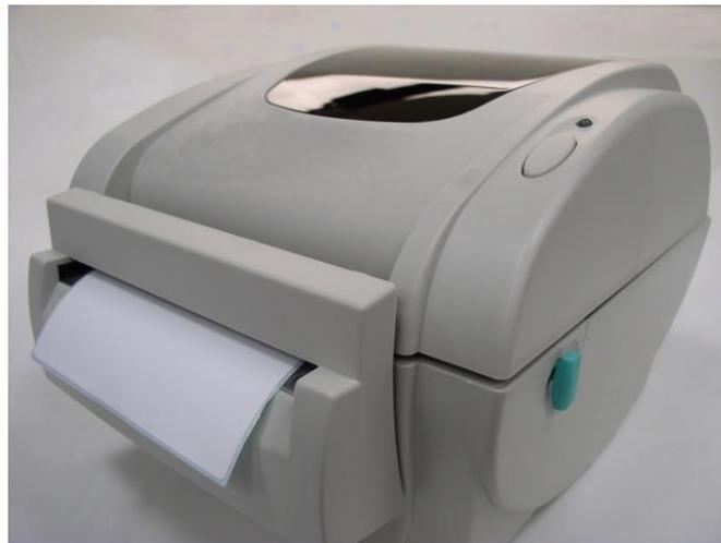
**Fig. 19 Media installation in cutter mode completed**
