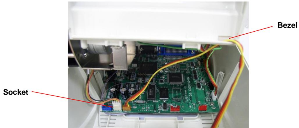
**Fig. 16 Cutter module harness arrangement**
