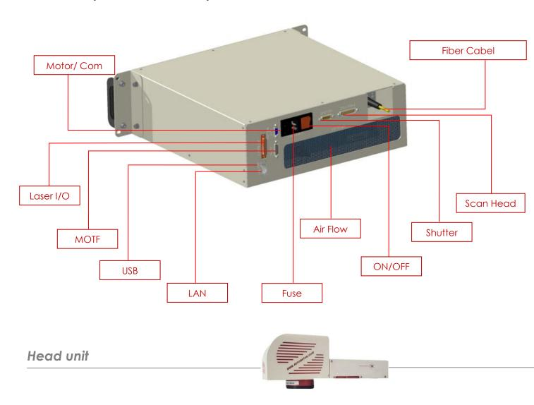
The head unit sets the galvanometric system and the lenses to focus the laser beam generated by the active fiber source in the Box unit.
